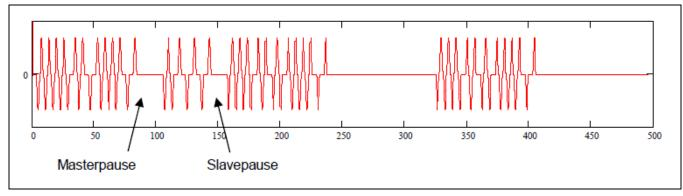
Figure 3.1 Test for SAP5 Revision C Error in Master Pause Detection
