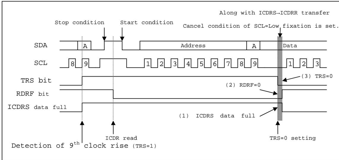
Figure 1. Notes on ICDR reading with TRS=1 setting in master mode.
