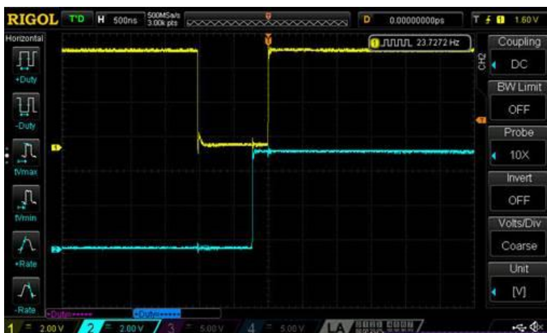
Figure 1. ACMP Output Glitch
