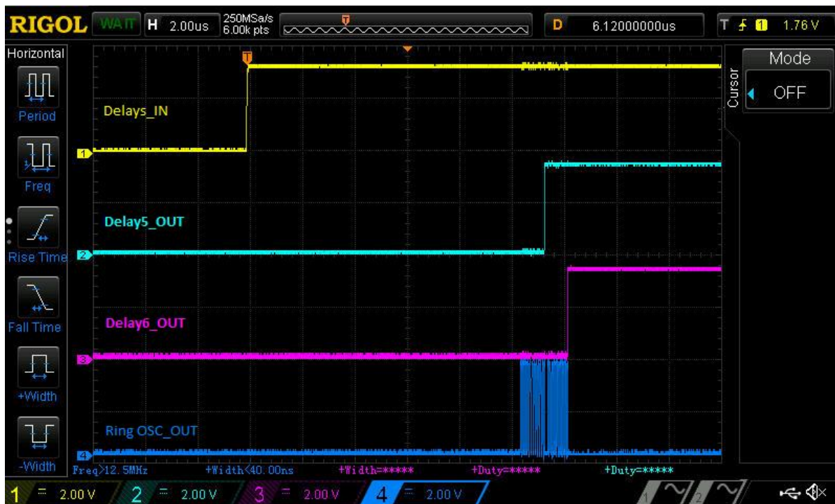
Figure 6. Ring OSC, DLY5 and DLY6 Waveform
