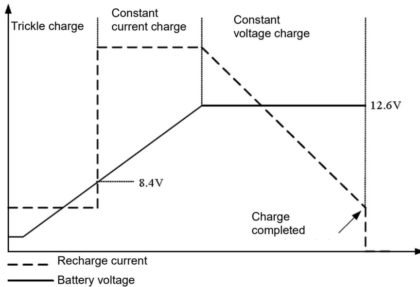
Figure 2. Charge current and voltage.
