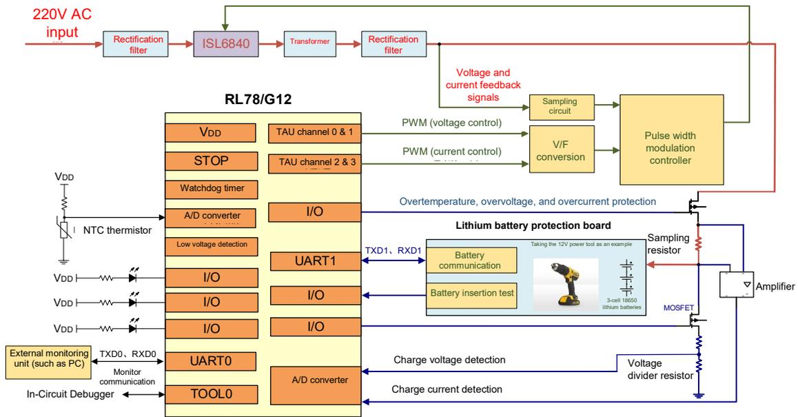
Figure 4. System block diagram
