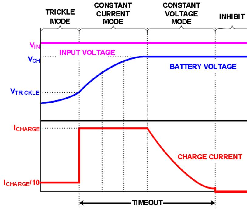
Figure 1. A typical charging curve for a lithium battery.
