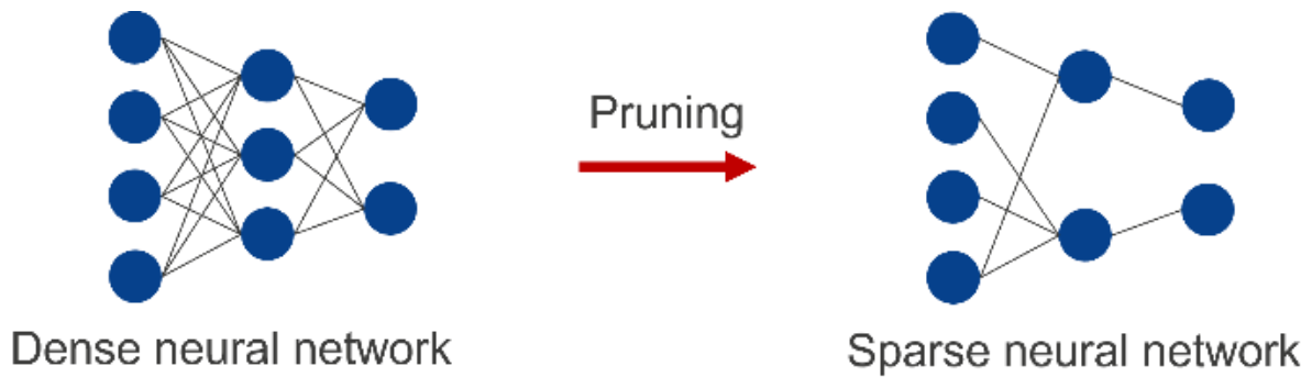
Figure 7: Reduction of Model Weight by Pruning
