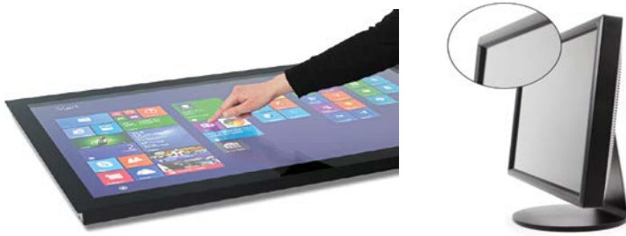
Figure 3: Tablet-like edge-to-edge compared to an IR-Touch based technology
