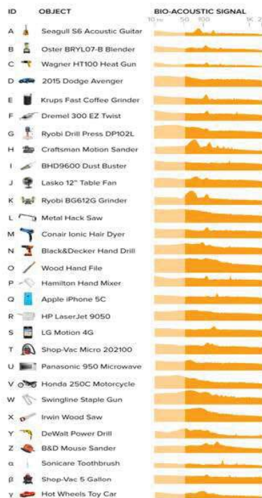
Illustration from the CMU study using vibrations captured with an overclocked smartwatch to detect what object a person is holding.
