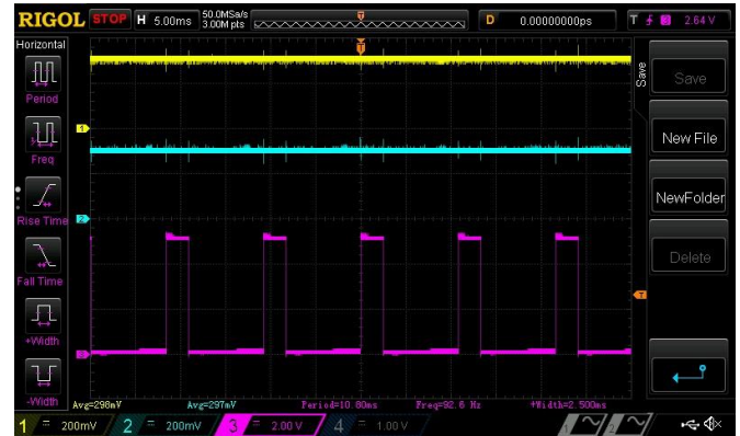
Fig 5. Timing waveforms for servomotor position 90 degrees
