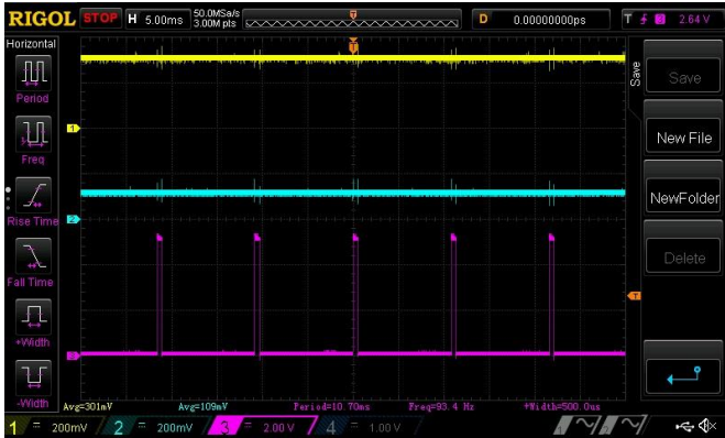
Fig 4. Timing waveforms for servomotor position -90 degrees
