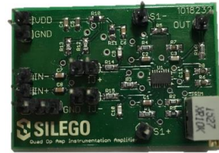
Figure 11. Instrumentation Amplifier PCB
