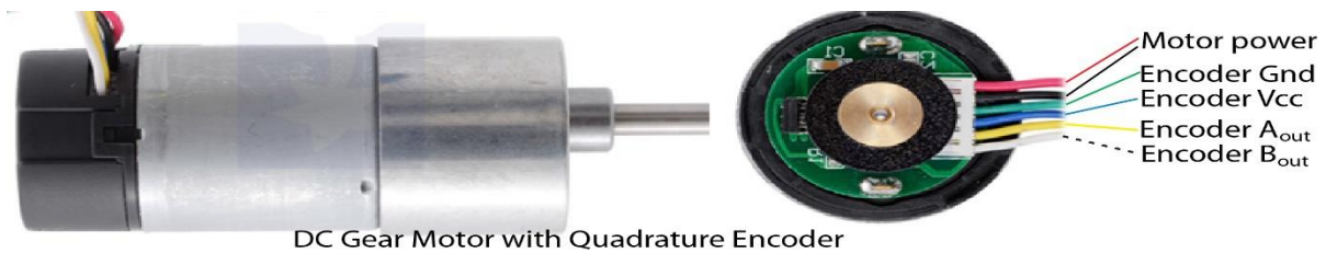
Figure 28: DC Gear Motor with Quadrature Encoder
