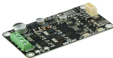
Figure 29: Cytron 10Amp DC Motor Driver
