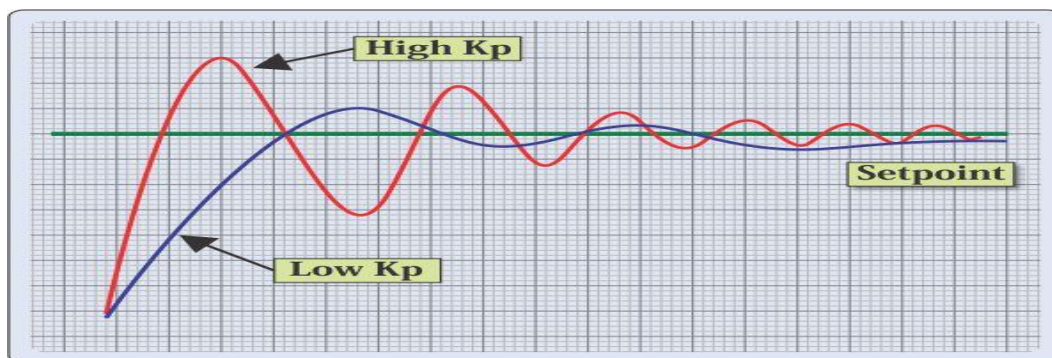
Figure 25: Reference Curves for P and I Parameters
