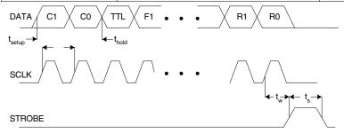
Figure 2. Timing Diagram for Programming the ICS307
