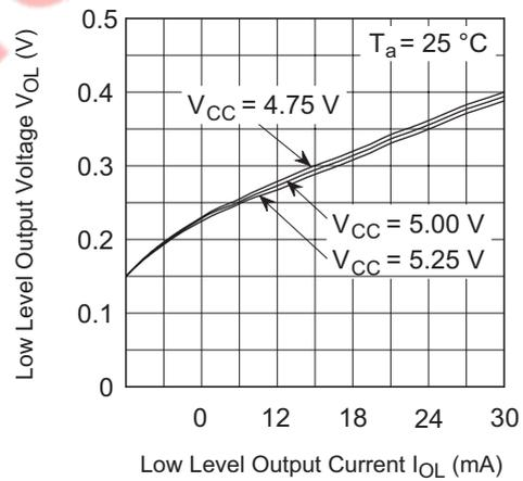
(e) Input / Output Characteristics at Receiver
