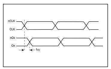
$Qx = t_{PW}$   $dc = \frac{t_{PW}}{t_{PERIOD}} \times 100\%$
