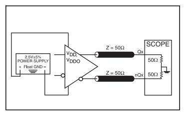
**LVDS Output Load AC Test Circuit**
