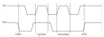
Figure 1: Standard I<sup>2</sup>C Transaction
