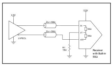
Figure 4C: IN/nIN Input with Built-In 50 $\Omega$  driven by an LVPECL Driver
