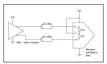
Figure 4B: IN/nIN Input with Built-In 50 $\Omega$  Driven by a CML Driver with Open Collector
