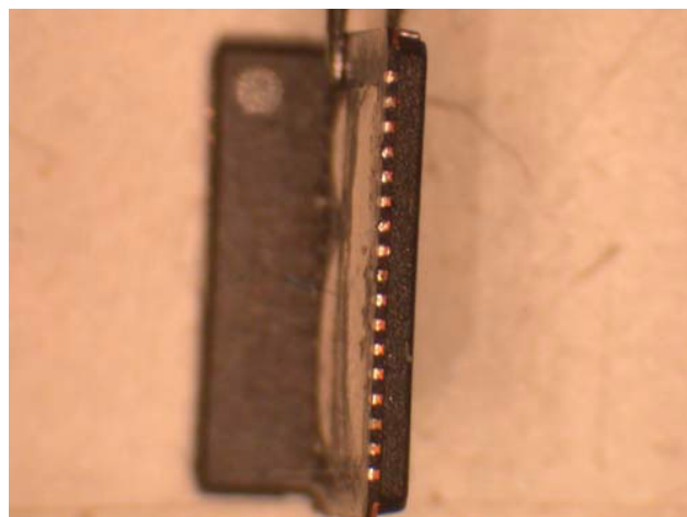
Figure 17. Finished Tinned Thermal Land on QFN
