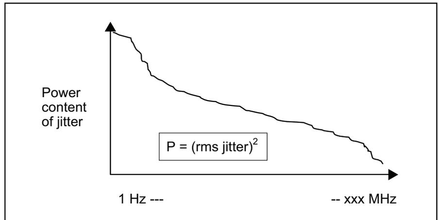
The area under the spectral density plot is related to the RMS jitter by:  $P = (\text{rms jitter})^2$
