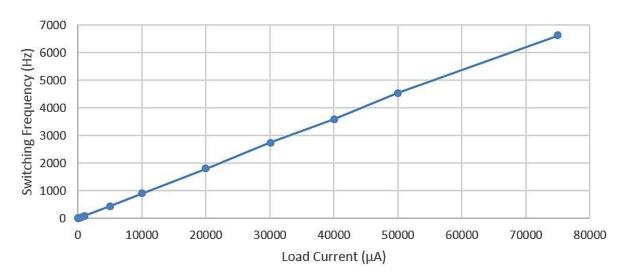
Figure 9: Load Current vs Switching Frequency, 10  $\mu A$  to 75 mA
