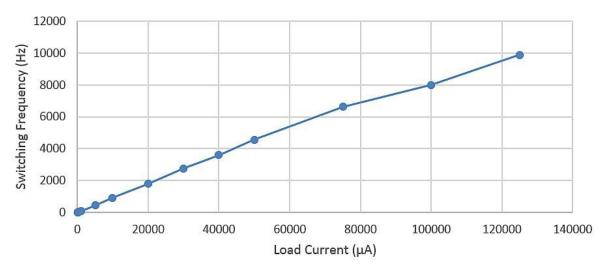
Figure 10: Load Current vs Switching Frequency, 10 μA to 125 mA
