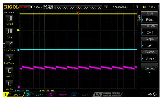
Figure 7: Operation at I\_LOAD = 50 μA
