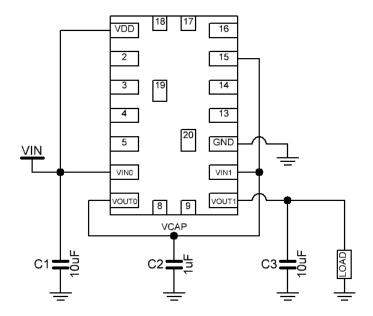
Figure 1: Circuit Diagram
