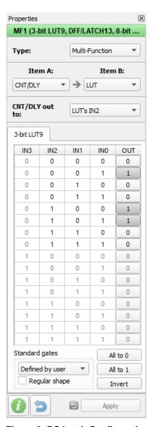
Figure 6: RS Latch Configuration
