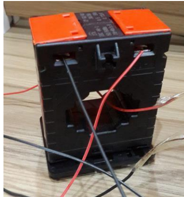
Figure 12. Ring main Current Transformer
