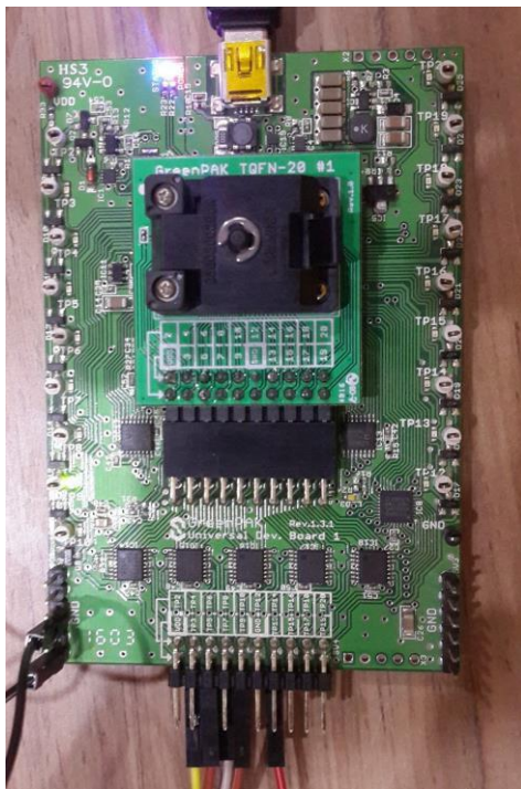
Figure 13. Normal Voltage (1V) LED Indication
