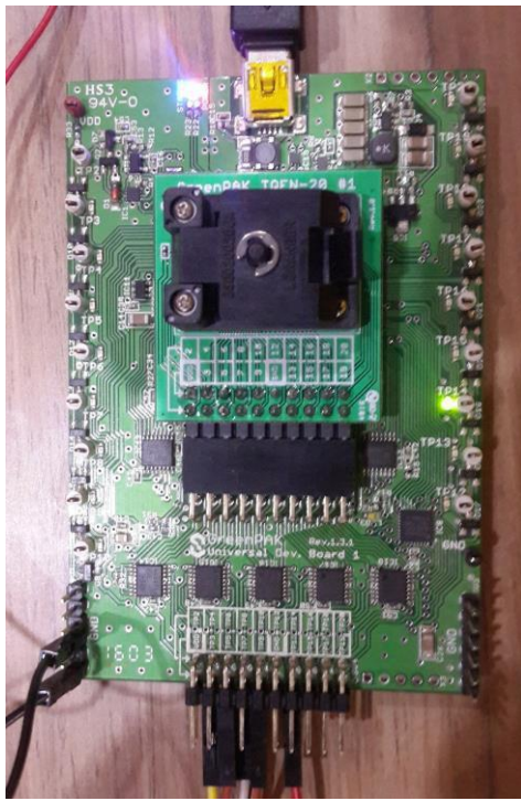
Figure 13. Normal Voltage (1V) LED Indication
