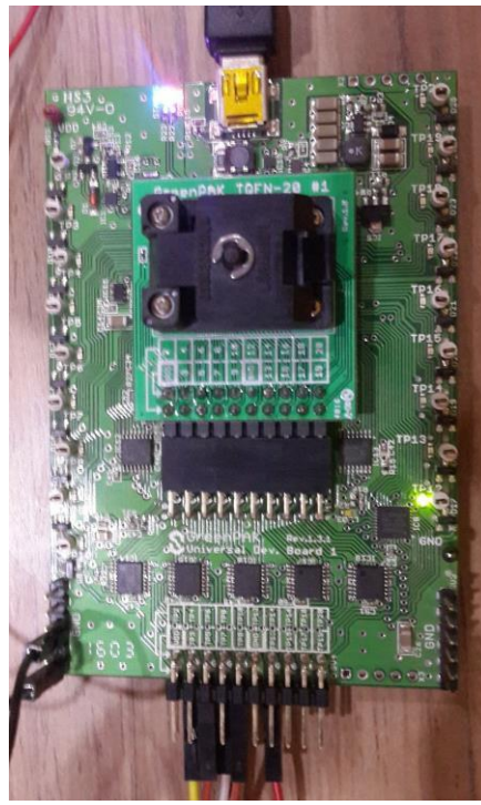
Figure 14. No Overload voltage ( 1.0 < V < 1.2 ) LED Indication
