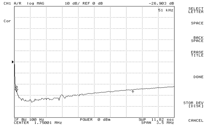
Figure-20 E1 120 Ω Receive Return Loss (Fully Internal Impedance Matching)
