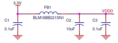
The ferrite bead above is any surface-mount bead with sufficient current rating for the circuits supplied. Please refer to AN-805 for ferrite bead recommendations.
