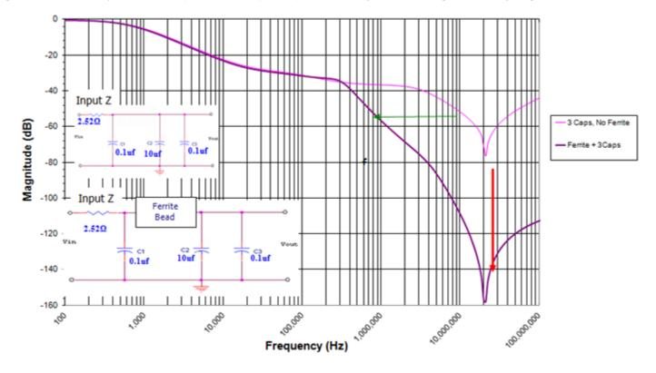
Figure 7. Noise Rejection Comparison: 0.1µF Capacitor Only vs Filtering Circuit by Figure 1
