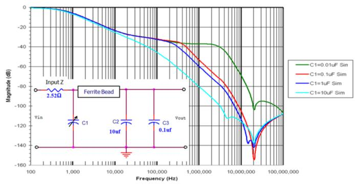
Figure 2. Sweeping C1 while keeping C2 =  $10\mu$ F, C3 =  $0.1\mu$ F
