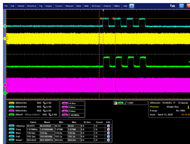
Figure 4. Waveform Sysref Limit Pulse Mode with Pulse Count = 4
