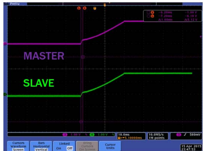
FIGURE 3. ISL8002B TRACKING START-UP
