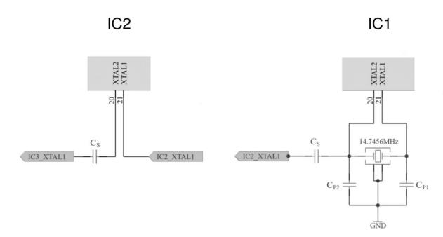
Figure 2. Crystal Oscillator Connection
