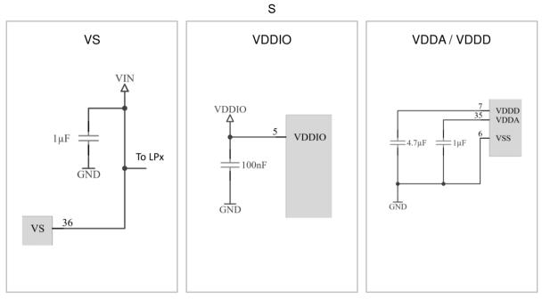
Figure 1. Power Supply Decoupling and Stabilization Network
