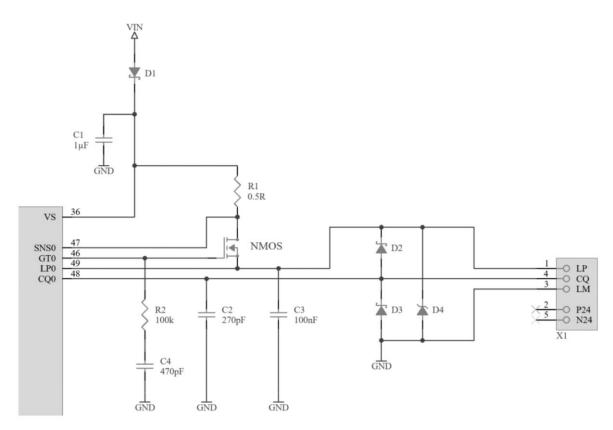
Figure 6. IO-Link Channel 0 Extended Circuitry
