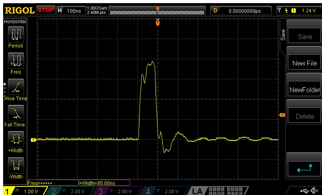
Figure 4: PIN3 Output Signal Zoomed in to Display 80 ns Pulse Width
