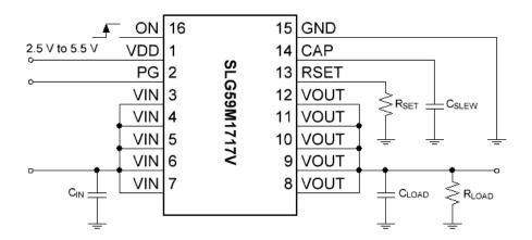
Figure 3: Typical Application Diagram of SLG59M1717V
