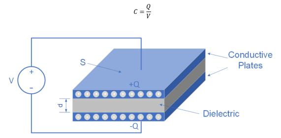
Figure 1: Two Charged Conductive Plates Separated with Dielectric Layer
