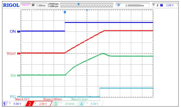
Figure 5: Typical Power up Operation Waveform for  $V_{DD} = V_{IN} = 4 V$ ,  $R_{SET} = 40 k\Omega$ ,  $C_{SLEW} = 10 nF$ ,  $R_{LOAD} = 100 \Omega$ ,  $C_{LOAD} = 10 \mu F$
