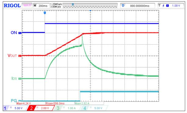
Figure 7: Typical Power Up for High Capacitive Load with Proper GreenFET Load Switch Slew Rate Settings for V<sub>DD</sub> = V<sub>IN</sub> = 4 V, I<sub>ACL</sub> = 5.7 A, R<sub>SET</sub> = 40 k $\Omega$ , C<sub>SLEW</sub> = 2  $\mu$ F, C<sub>LOAD</sub> = 0.66 F, R<sub>LOAD</sub> = 100  $\Omega$
