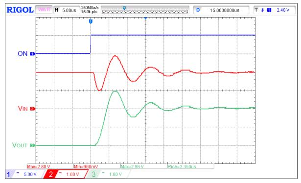
Figure 9. A Fast, Nanopower Load Switch Powering Up a 10 µF Load Capacitor.
