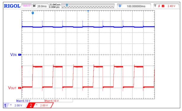
Figure 12. The Parasitic Inductance of 1.2-m Length AWG13 Wires from Power Supply Causes Voltage Spikes at V<sub>IN</sub> during Active Current Limit Operation.
