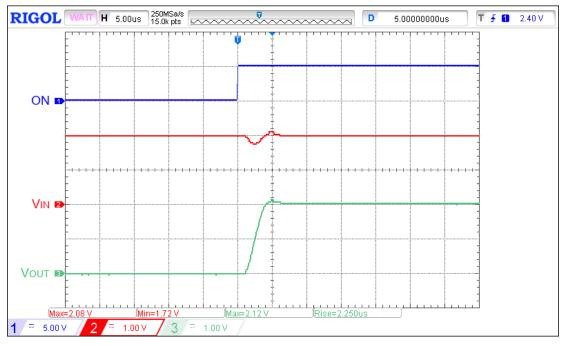
Figure 10. A Fast, Nanopower Load Switch Powering Up a 10 μF Load Capacitor with a 1000 μF Aluminum Electrolytic Capacitor at VIN (C<sub>IN</sub>).
