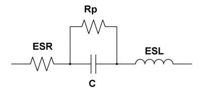
Figure 1. Capacitor Equivalent Circuit
