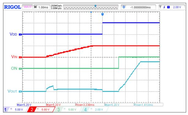
Figure 5. Powering Up a Load Switch when V<sub>IN</sub> is Applied Before V<sub>DD</sub>.
