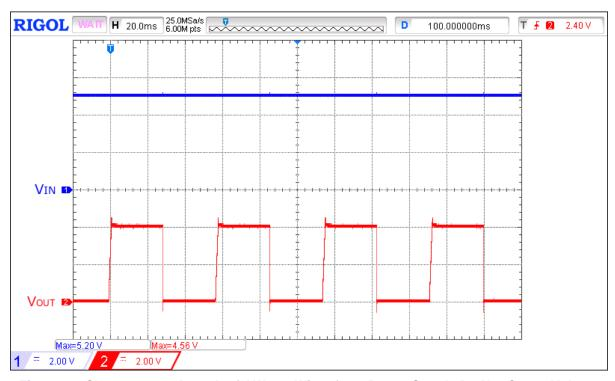
Figure 13. Shorter, 0.2-m Length of AWG13 Wires from Power Supply Do Not Cause Voltage Spikes at V<sub>IN</sub> during Active Current Limit Operation.
