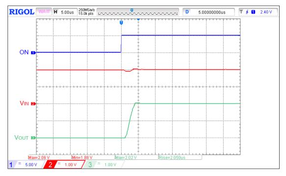
Figure 11. A Fast, Nanopower Load Switch Powering up a 10 μF Load Capacitor with a 270 μF Low ESR/ESL Aluminum Polymer Input Capacitor at VIN (C<sub>IN</sub>).
