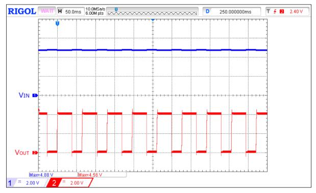
Figure 14. Adding 470 µF Low ESR/ESL Aluminum Polymer Capacitor at VIN Eliminates Voltage Spikes Caused by the Parasitic Inductance of the 1.2-m Length AWG13 Wires from Power Supply during Active Current Limit Operation.
