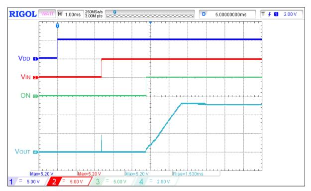
Figure 3. Powering Up a Load Switch with Fast  $V_{\text{DD}}$  and  $V_{\text{IN}}$  Rise Times.
