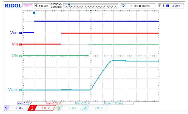
Figure 6. A Load Switch Powering Up a 1 μF Load Capacitor with Fast V<sub>DD</sub> and V<sub>IN</sub> rise Times.
