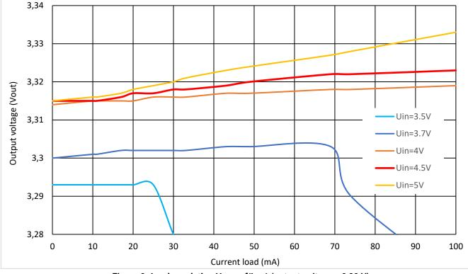
Figure 9: Load regulation VOUT = f(IOUT) (output voltage = 3.30 V)
