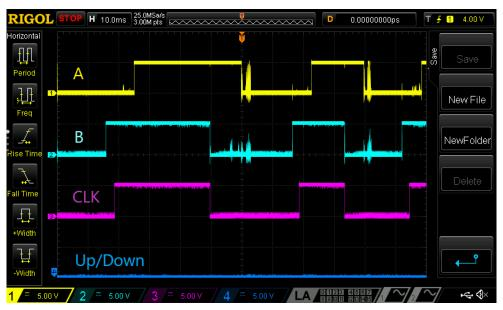
Figure 5: Timing Diagrams for Counterclockwise Encoder Rotation
