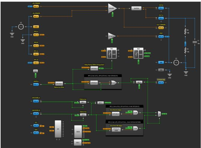
This design is similar to the previous one. It has the same encoder management logic. The differences in this design are due to the analog parts. The design allows you to adjust the voltage in the range from 0 V to 4.0 V, unlike the previous one, whose adjustment range is from 0.5 V to 4.5 V. Another difference of this design is that when the encoder button is pressed for a long time, the output voltage is reduced to zero.
