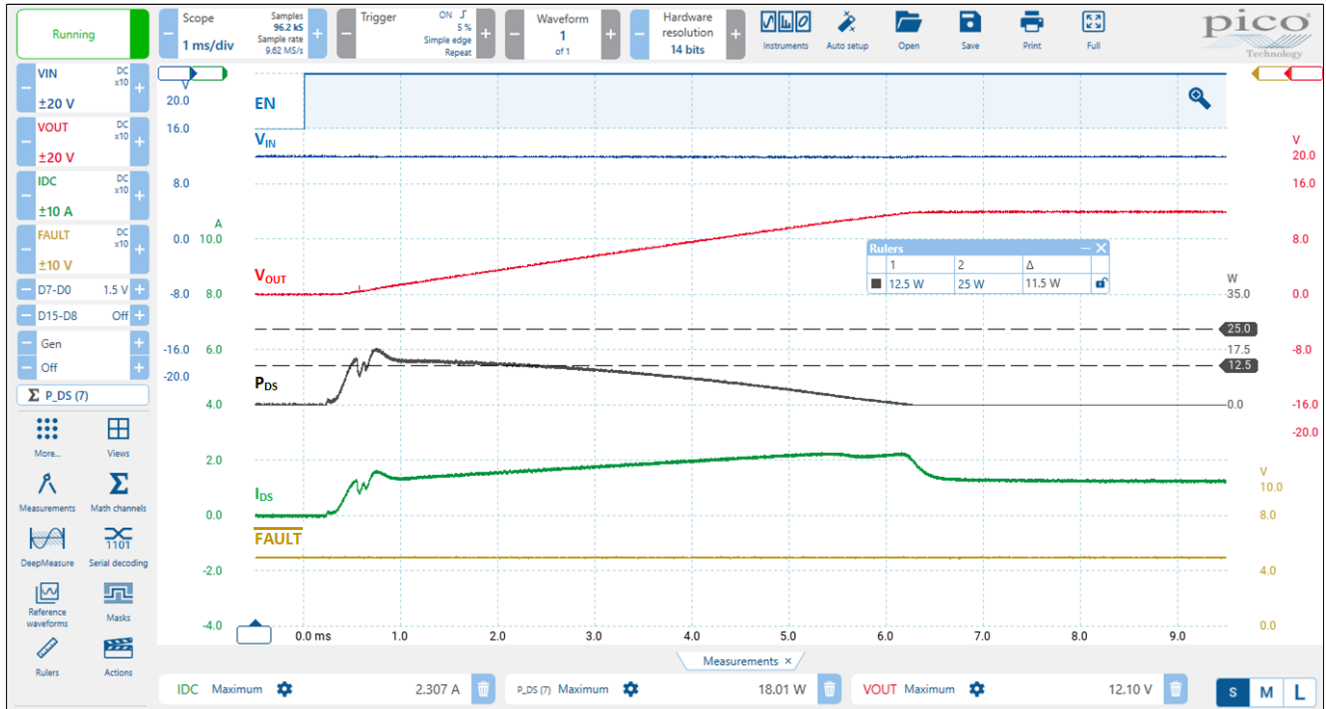
Figure 21. Turn-on operation waveform for V_{IN} = 12 \text{ V} , C_{SLEW} = 16 \text{ nF} , R_{SET} = 14 \text{ k}\Omega , C_{LOAD} = 600 \text{ }\mu\text{F} , R_{LOAD} = 10 \text{ }\Omega
