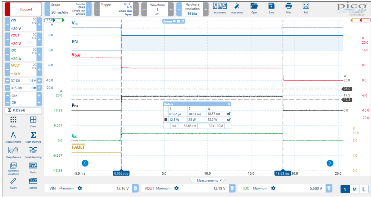
Figure 14: SLG59H1132V 12.5 W SOA operating waveform during Active Current Limit for V_{IN} = 12\text{ V} , C_{SLEW} = 10\text{ nF} , R_{SET} = 30.1\text{ k}\Omega , C_{LOAD} = 10\text{ }\mu\text{F} , R_{LOAD} = \text{switch in } 2\text{ }\Omega (Extended view)
