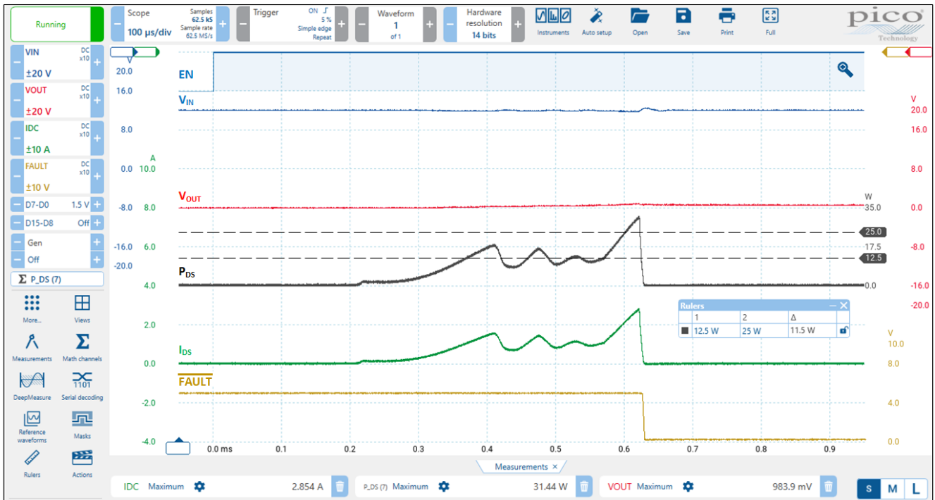
Figure 20. Turn-on operation waveform for V_{IN} = 12\text{ V} , C_{SLEW} = 10\ \text{nF} , R_{SET} = 14\ \text{k}\Omega , C_{LOAD} = 600\ \mu\text{F} , R_{LOAD} = 10\ \Omega
