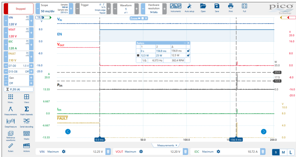
Figure 15: SLG59H1132V 25 W SOA operating waveform during Active Current Limit for V_{IN} = 12\text{ V} , C_{SLEW} = 10\text{ nF} , R_{SET} = 30.1\text{ k}\Omega , C_{LOAD} = 10\text{ }\mu\text{F} , R_{LOAD} = \text{switch in } 1\text{ }\Omega
