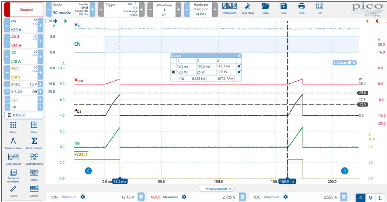
Figure 7: SLG59H1132V 25 W SOA operation waveform for V_{IN} = 12\text{ V} , ON = \text{Low} \rightarrow \text{High} , C_{SLEW} = 150\text{ nF} , R_{SET} = 14\text{ k}\Omega , C_{LOAD} = 10\text{ }\mu\text{F} , R_{LOAD} = 1\text{ }\Omega
