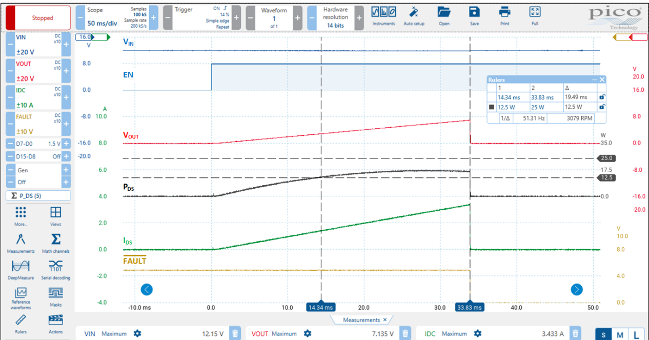
Figure 10: SLG59H1132V 12.5 W SOA operating waveform for V_{IN} = 12\text{ V} , ON = Low \rightarrow High, C_{SLEW} = 150\text{ nF} , R_{SET} = 14\text{ k}\Omega , C_{LOAD} = 10\text{ }\mu\text{F} , R_{LOAD} = 2\text{ }\Omega (Extended view)
