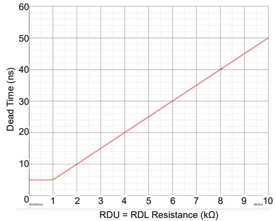
Figure 3. Dead Time vs RDU/RDL Resistor (Simulation)
