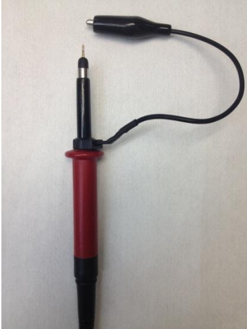
Fig.6. Typical probe with 3-inch ground lead – should not be used
