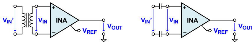
Figure 6. AC-Coupling Removes the Ground Reference of the Original Input Signal, V_{IN}' , so that V_{IN} is Floating
