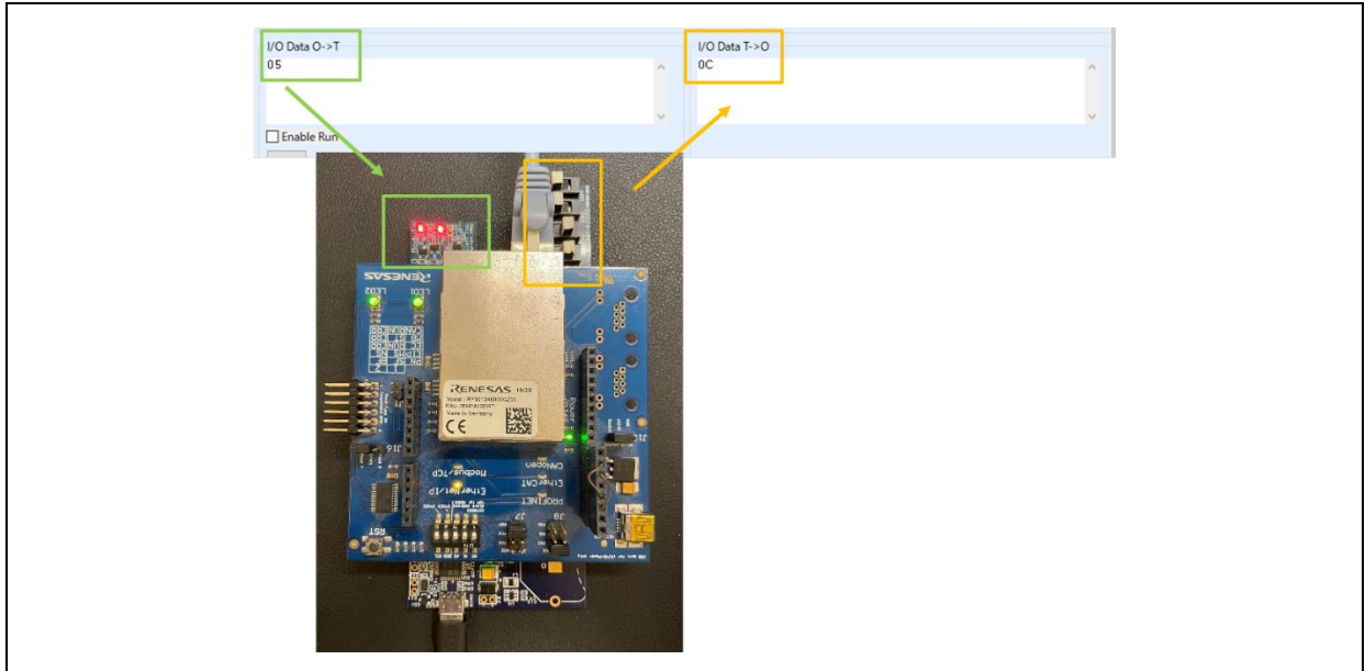
図 3-43 Remote-IO (LED/Switch)制御 [EtherNet/IP]
