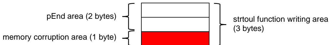
Figure 9-4 Memory corruption due to example of W0520167
