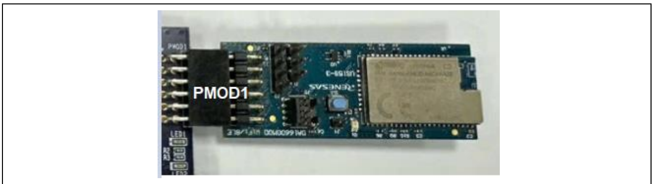
Figure 4-2 Connecting DA16600MOD to PMOD1 of the MCU Board
