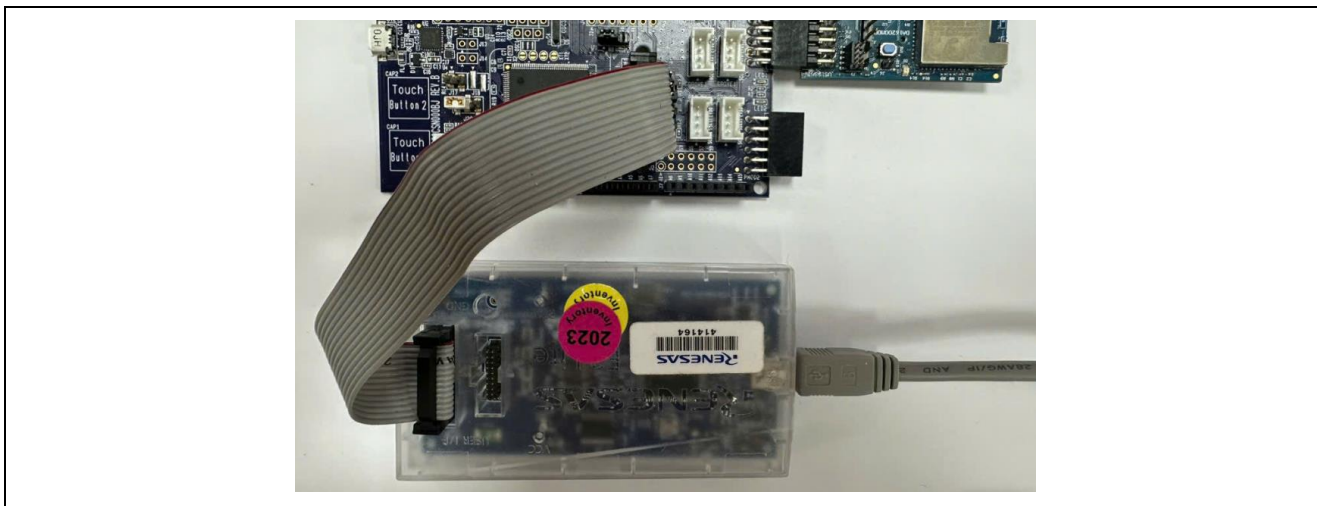
Figure 8-5 Connecting Emulator to MCU Board
