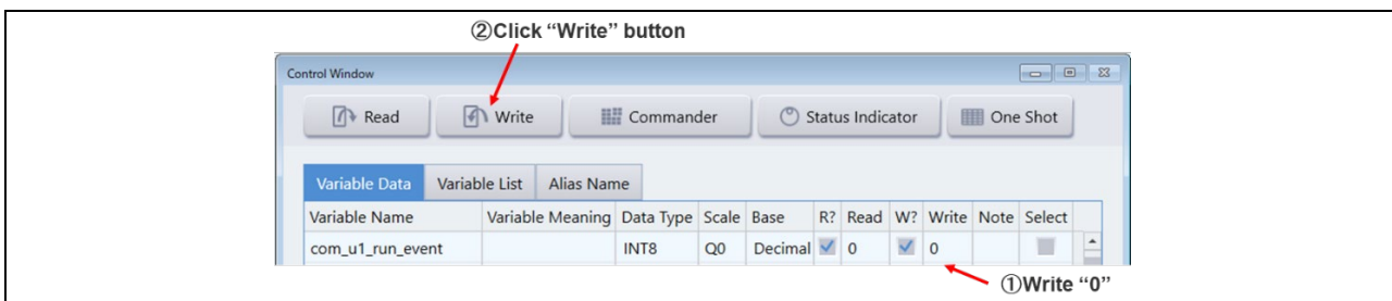
Figure 4-3 Procedure - Stop the motor
