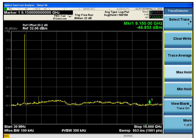
Figure 23 TX Spurious emission (Frequency = 915.2MHz)
