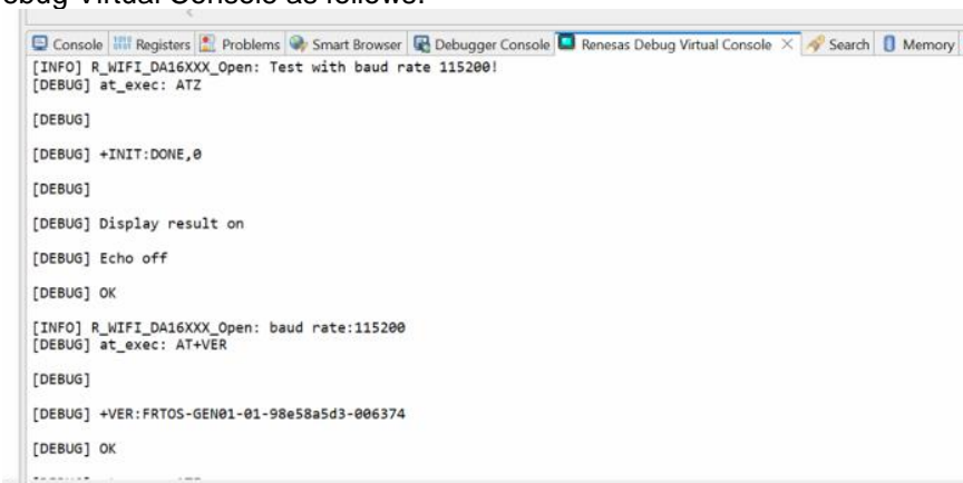
Figure 6.7 Wi-Fi Logging on Renesas Debug Virtual Console
