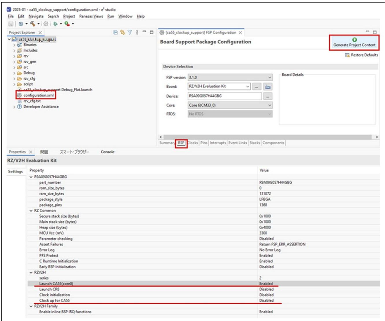
Figure 3-3. CM33 project setting for CM33 cold boot
