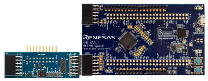
Figure 8. RA MCU and QCIOT Board Connection
