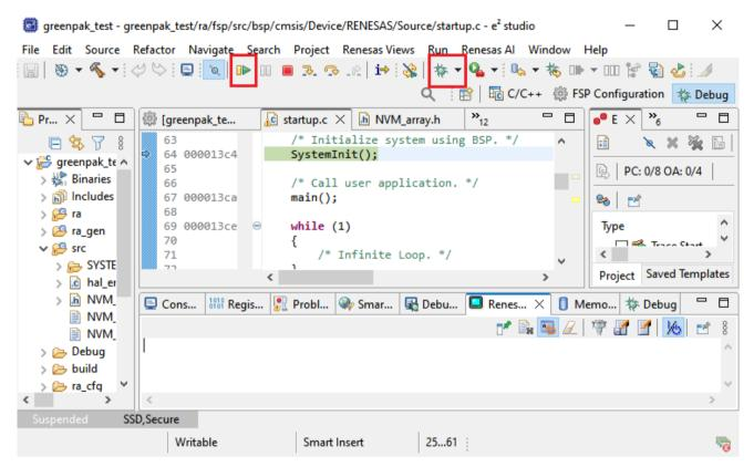
Figure 9. Flash and Run the Code
