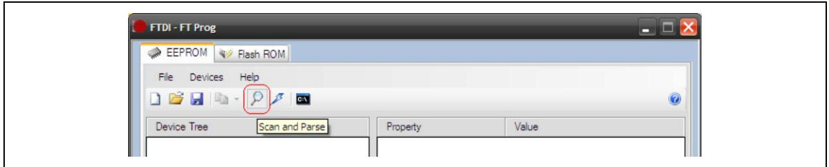
Figure 4.3 Searching for the Connected SSC Communication Board
