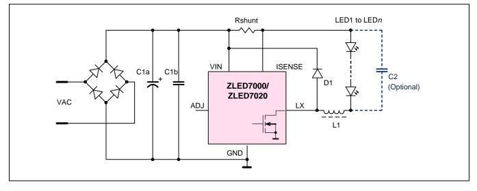
Figure 7.1 AC Operation of the ZLED7000 or ZLED7020
