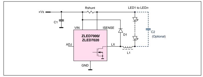
The current levels for the power transistor to turn on and off are determined by the voltage drop across Rshunt. An internal hysteresis comparator detects this voltage with an initial threshold of 95 mV (typical) with a symmetrical  $\pm$  15% hysteresis. The average LED current is defined as
