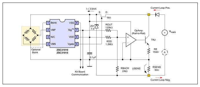
Figure 2.1 – ZSC31010 with Current Loop Output Using ZACwire™ Communication
