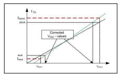
This transfer function for the measured currents  $I_{4mA}$  and  $I_{20mA}$  is given by
