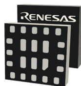
2.0 mm x 2.2 mm 22-pin MSTQFN 0.4 mm pitch
