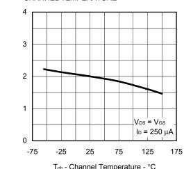
Vcs(th) - Gate to Source Threshold Voltage - V
