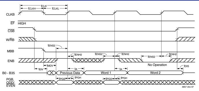
Figure 4. FIFO Read Cycle Timing
