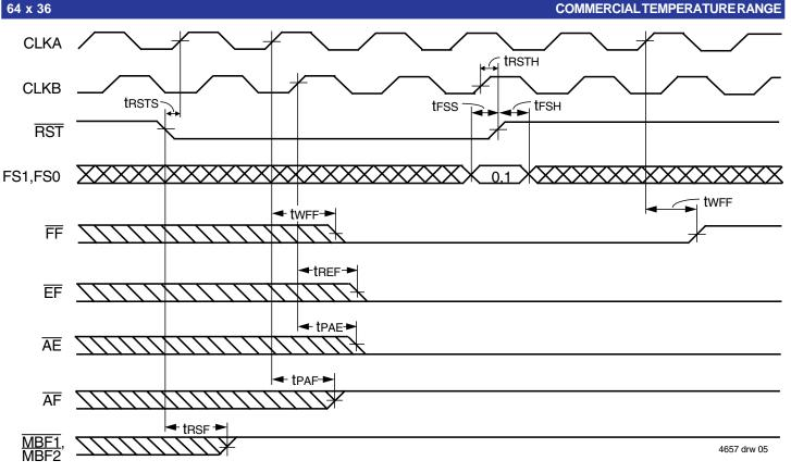
Figure 2. Device Reset and Loading the X Register with the Value of Eight
