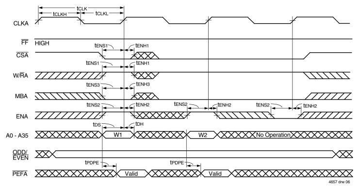
Figure 3. FIFO Write Cycle Timing
