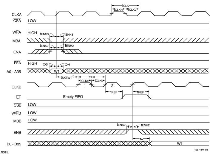
1. tskew1 is the minimum time between a rising CLKA edge and a rising CLKB edge for  $\overline{\mathsf{EF}}$  to transition HIGH in the next CLKB cycle. If the time between the rising CLKA edge and rising CLKB edge is less than tskew1, then the transition of  $\overline{\mathsf{EF}}$  HIGH may occur one CLKB cycle later than shown.
