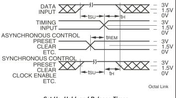
Set-Up, Hold, and Release Times
