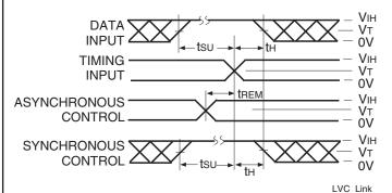
Set-up, Hold, and Release Times
