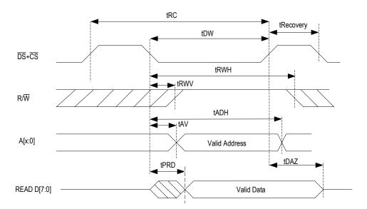
Figure-34 Non-Multiplexed Motorola Read Timing
