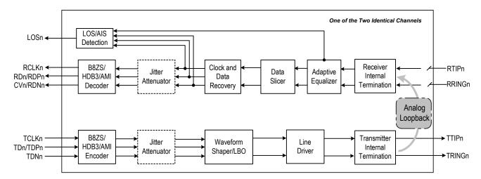
Figure-15 Analog Loopback
