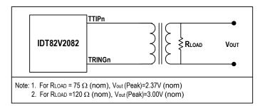
Figure-5 E1 Pulse Template Test Circuit
