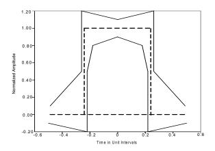
Figure-4 E1 Waveform Template Diagram
