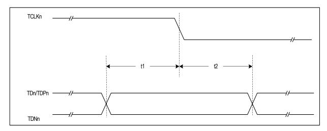
Figure-24 Transmit System Interface Timing
