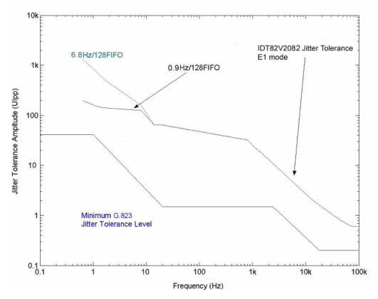
Figure-26 E1 Jitter Tolerance Performance
