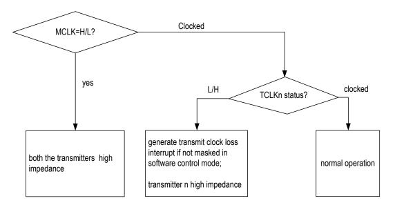
Figure-20 TCLK Operation Flowchart
