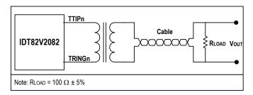
Figure-7 T1 Pulse Template Test Circuit
