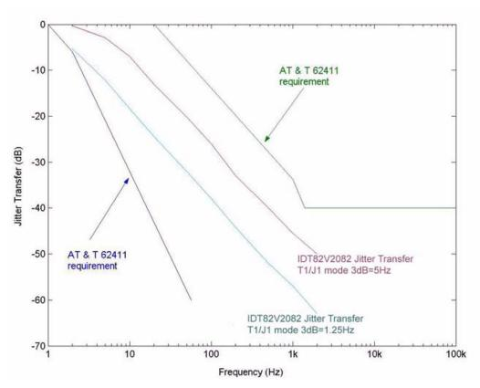
Figure-29 T1/J1 Jitter Transfer Performance
