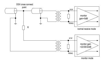
Figure-10 Monitoring Receive Line in Another Chip
