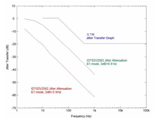
Figure-28 E1 Jitter Transfer Performance
