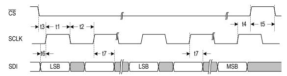
Figure-31 Serial Interface Write Timing
