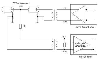
Figure-11 Monitor Transmit Line in Another Chip
