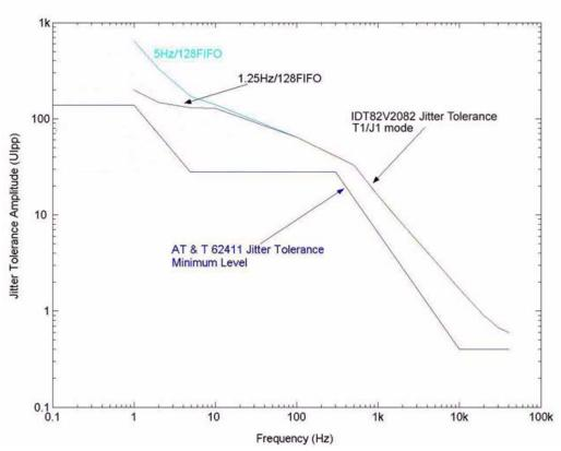
Figure-27 T1/J1 Jitter Tolerance Performance
