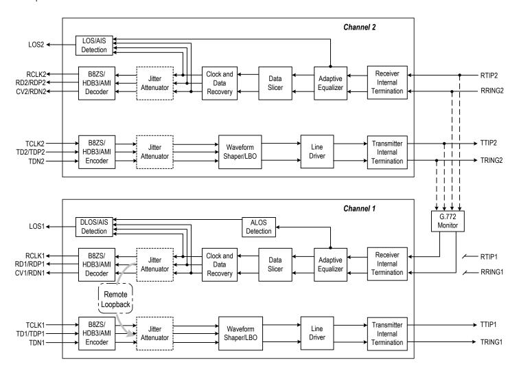
Figure-12 G.772 Monitoring Diagram
