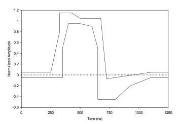
Figure-6 DSX-1 Waveform Template
