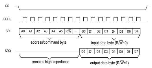
Figure-21 Serial Microcontroller Interface Function Timing
