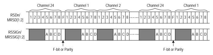
Figure 8. Signaling Output in T1/J1 Mode
