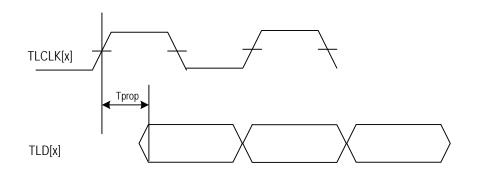
Figure 94. Transmit Line Interface Timing
