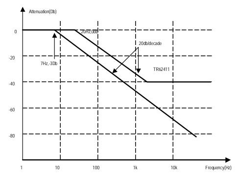
Figure 68. T1/J1 Mode Jitter Transfer (N1 = N2 = 2fH)
