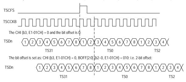
Figure 48. Transmit Bit Offset in E1 Mode - 1
