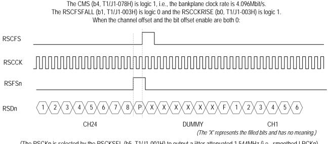
(The RSCKn is selected by the RSCKSEL (b5, T1/J1-001H) to output a jitter attenuated 1.544MHz (i.e., smoothed LRCKn) or 8KHz clock (smoothed LRCKn divided by 193).)
