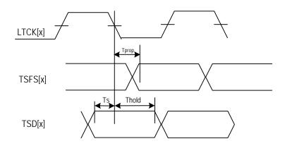
Figure 90. Transmit Interface Timing (Line Transmit Clock)
