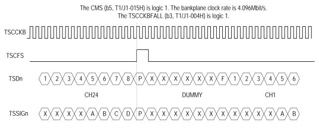
Figure 59. T1/J1 Transmit Clock Slave External Signaling Mode - Functional Timing Example 3
