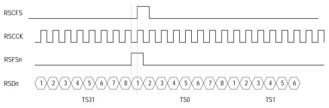
(The RSCKn is selected by the RSCKSEL (b5, E1-001H) to output a jitter attenuated 2.048MHz (i.e., smoothed LRCKn) or 8KHz clock (smoothed LRCKn divided by 256).)
