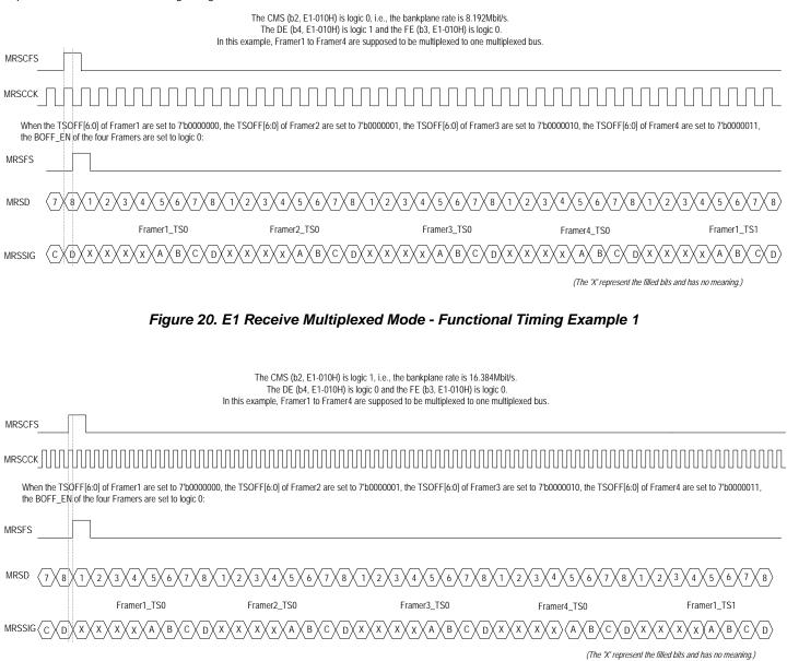
Figure 21. E1 Receive Multiplexed Mode - Functional Timing Example 2
