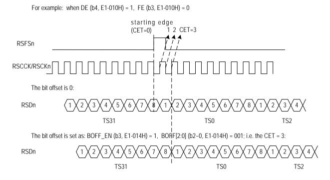
Figure 23. Receive Bit Offset - Between RSFSn & RSDn
