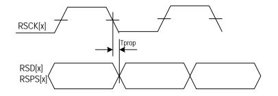
Figure 92. Receive Interface Timing (Receive System Clock)
