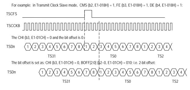
Figure 49. Transmit Bit Offset in E1 Mode - 2
