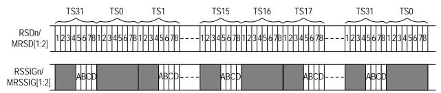
Figure 7. Signaling Output in E1 Mode
