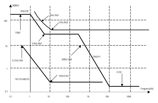
Figure 67. T1/J1 Mode Jitter Tolerance (N1 = N2 = 2fH)
