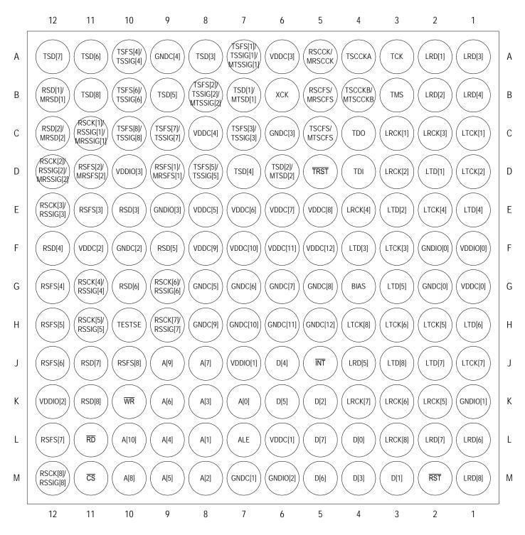
Figure 2. 144-Pin PBGA (Bottom View)
