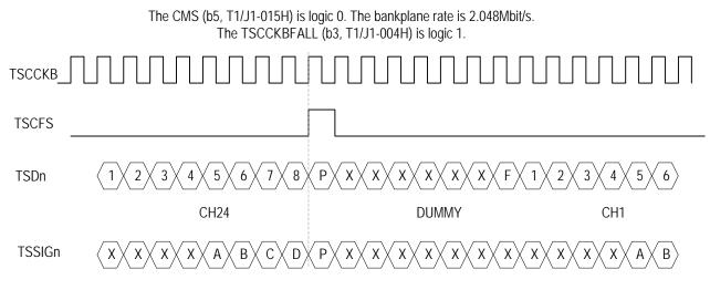
Figure 58. T1/J1 Transmit Clock Slave External Signaling Mode - Functional Timing Example 2
