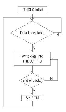
Figure 80. Writing Data to T1/J1 Mode THDLC FIFO
