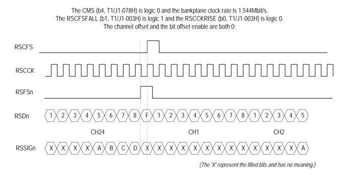
Figure 28. T1/J1 Receive Clock Slave External Signaling Mode - Functional Timing Example 1
