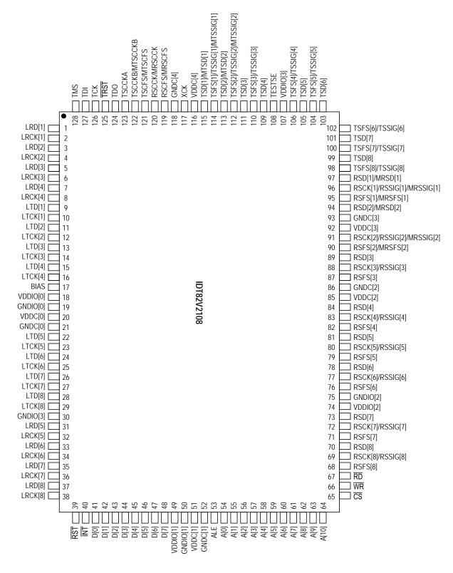
Figure 1. 128-Pin PQFP (Top View)
