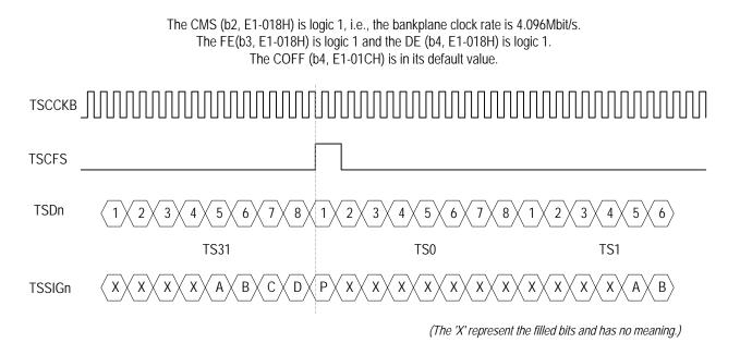
Figure 42. E1 Transmit Clock Slave External Signaling Mode - Functional Timing Example 2
