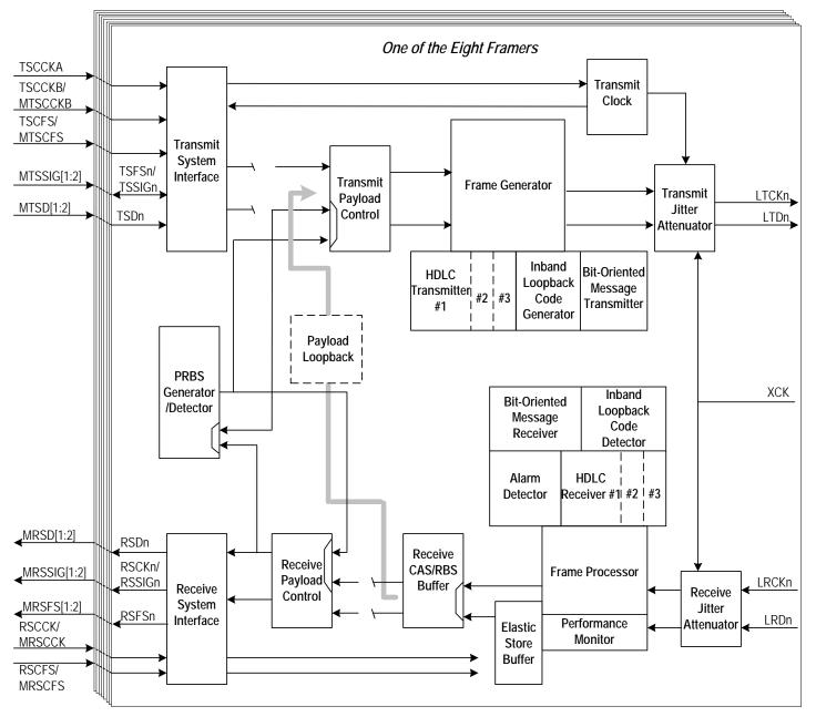
Figure 72. Payload Loopback
