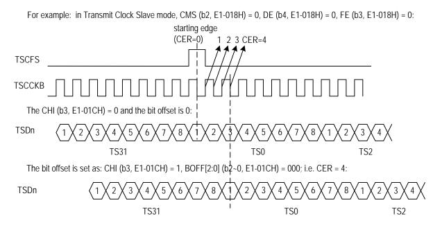
Figure 50. Transmit Bit Offset in E1 Mode - 3
