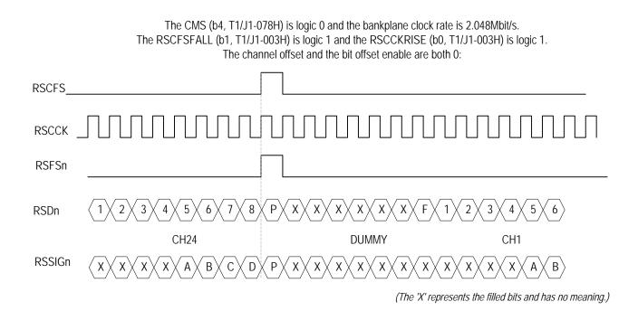
Figure 29. T1/J1 Receive Clock Slave External Signaling Mode - Functional Timing Example 2
