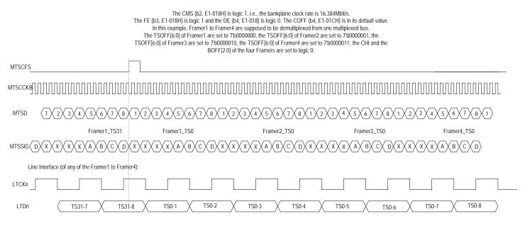
Figure 47. E1 Transmit Multiplexed Mode - Functional Timing Example 2
