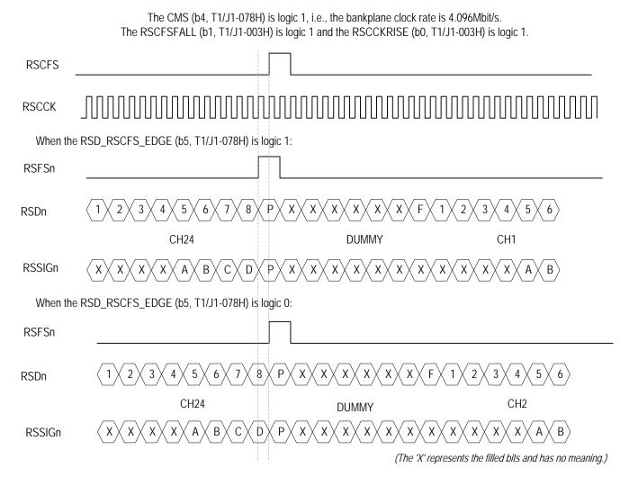
Figure 30. T1/J1 Receive Clock Slave External Signaling Mode - Functional Timing Example 3
