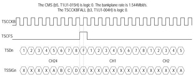
Figure 57. T1/J1 Transmit Clock Slave External Signaling Mode - Functional Timing Example 1
