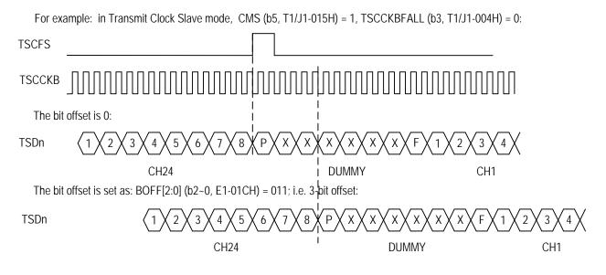
Figure 64. Transmit Bit Offset in T1/J1 Mode - 2
