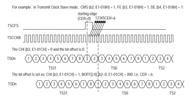
Figure 51. Transmit Bit Offset in E1 Mode - 4
