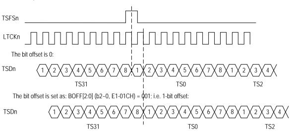
For example: in Transmit Clock Master mode, DE (b4, E1-018H) = 1, TSFSRISE (b2, E1-002H) = 1:
