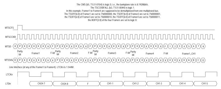
Figure 61. T1/J1 Transmit Multiplexed Mode - Functional Timing Example 1
