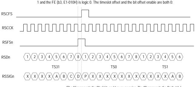
The CMS (b2, E1-010H) is logic 0, i.e., the bankplane rate is 2.048Mbit/s. The DE (b4, E1-010H) is logic 1 and the FE (b3, E1-010H) is logic 0. The timeslot offset and the bit offset enable are both 0:
