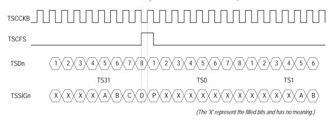
Figure 41. E1 Transmit Clock Slave External Signaling Mode - Functional Timing Example 1
