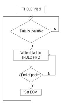
Figure 74. Writing Data to E1 Mode THDLC FIFO
