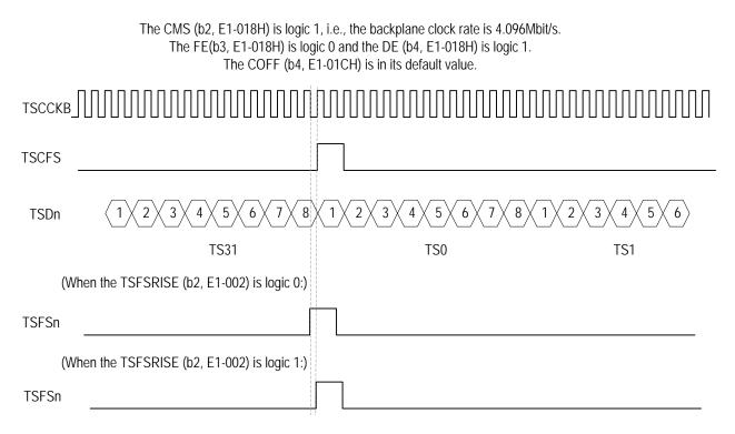
Figure 39. E1 Transmit Clock Slave TSFS Enable Mode - Functional Timing Example 2
