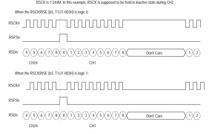
Figure 32. T1/J1 Receive Clock Master Fractional T1/J1 Mode - Functional Timing Example
