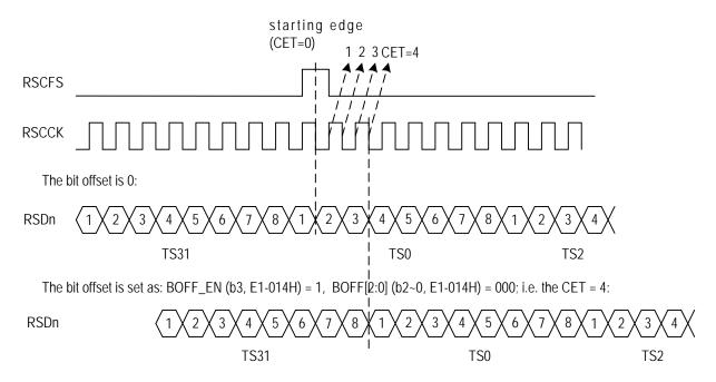
Figure 22. Receive Bit Offset - Between RSCFS & RSDn
