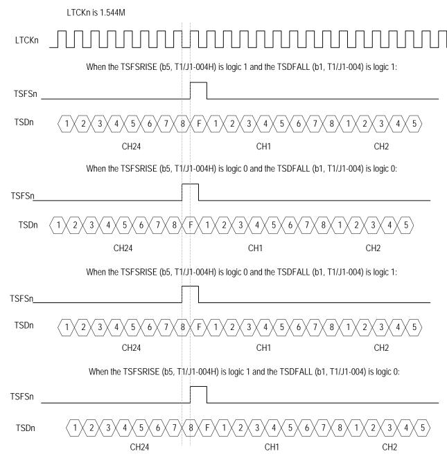
Figure 60. T1/J1 Transmit Clock Master Mode - Functional Timing Example
