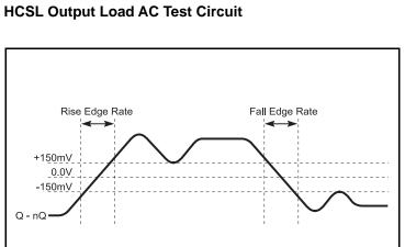
Differential Measurement Points for Rise/Fall Edge Rate
