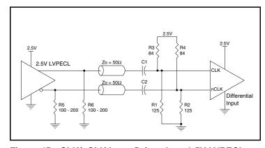
Figure 4D. CLK/nCLK Input Driven by a 2.5V LVPECL Driver with AC Couple
