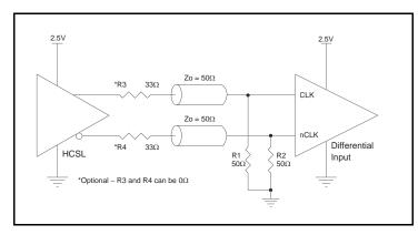
Figure 4B. CLK/nCLK Input Driven by a 2.5V HCSL Driver
