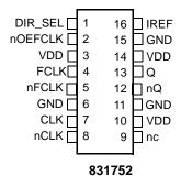
16-lead TSSOP 4.4mm x 5.0mm x 0.925mm package body G Package, Top View
