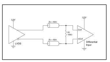
Figure 4E. CLK/nCLK Input Driven by a 2.5V LVDS Driver
