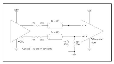
Figure 3B. CLK/nCLK Input Driven by a 3.3V HCSL Driver
