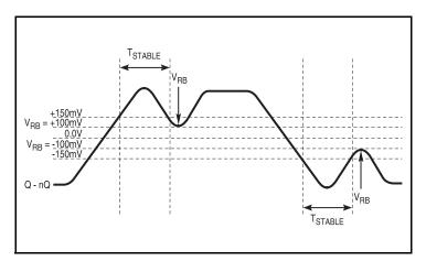
**Differential Measurement Points for Ringback**
