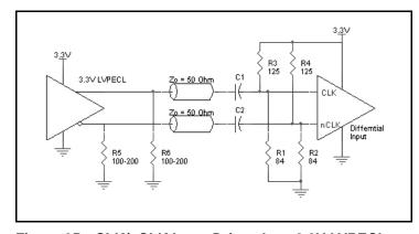
Figure 3D. CLK/nCLK Input Driven by a 3.3V LVPECL Driver with AC Couple
