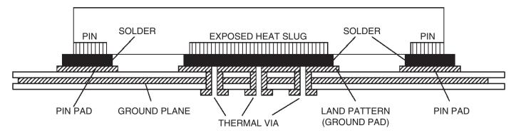
Figure 6. P.C. Assembly for Exposed Pad Thermal Release Path – Side View (drawing not to scale)
