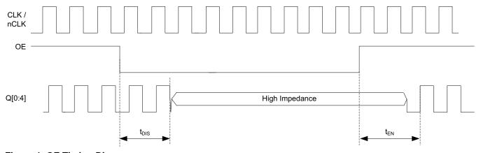
Figure 1. OE Timing Diagram
