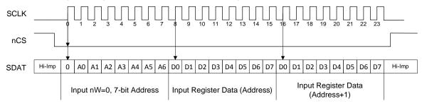
Table 24. SPI Read / Write Cycle Timing Parameters
